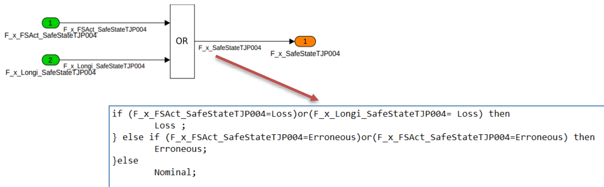
Figure 10. Transition from Simulink logics to AltaRica assertions
