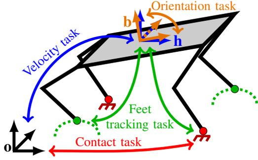
Fig. 3: Tasks and frames of the WBC.
