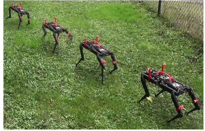
Fig. 11: Trotting gait on wet grass. Connection with the robot was done by Wifi with the same computer than we used indoors. Previous experiments showed that packet loss did not hamper the behavior for distance under 25 m.
