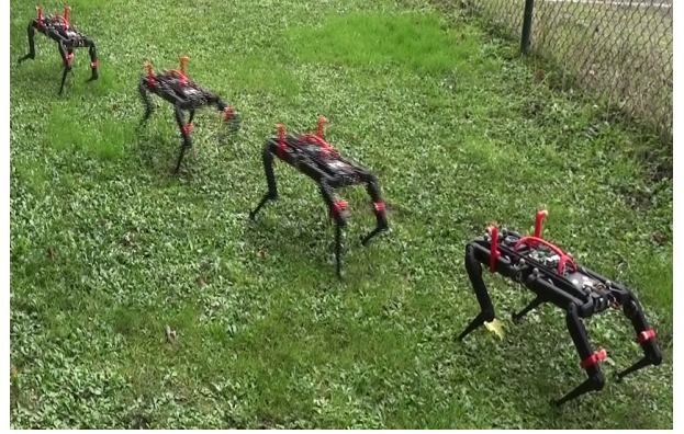
Fig. 10: Trotting gait on wet grass. Connection with the robot was done by Wifi with the same computer than we used indoors. Previous experiments showed that packet loss did not hamper the behavior for distance under 25 m.
