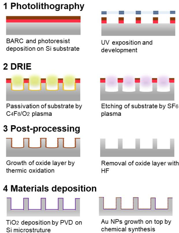
**Figure 2.** Main process steps underlining the cross-section of the 3D photocatalyst: (1) photolithography; (2) deep reactive ion etching where consecutive cycles of  $SF_6$  and  $C_4F_8/O_2$  steps etch and passivate the silicon; (3) postprocessing by thermal oxidation of silicon followed by the removal of the oxide layer; and (4)  $TiO_2$  layer sputter deposition followed by (optional) chemical synthesis of Au nanoparticles.
