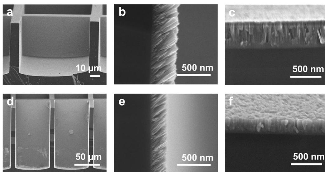
**Figure 8.** SEM cross-sectional images of the 3D photocatalyst composed of silicon microstructures and TiO<sub>2</sub> film, corresponding to samples A3-T2 (a-c) and A7-T2 (d-f) featuring AEFs of 3 and 7, respectively. Details of the compact TiO<sub>2</sub> layer at half-heights of the wall (b, e) and bottom of the microcavities (c, f).
