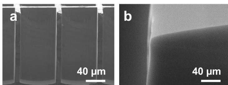
**Figure 6.** SEM cross-section images of silicon microstructures after postprocessing: details of several microcavities (a) and a magnified view of an upper wall corner (b). DRIE process SF<sub>6</sub> and C<sub>4</sub>F<sub>8</sub>/O<sub>2</sub> exposure times of 1.5 and 2.0 s, respectively. The measured geometrical parameters are depth = 156 μm, w = 75 μm and a = 10.4 μm.
