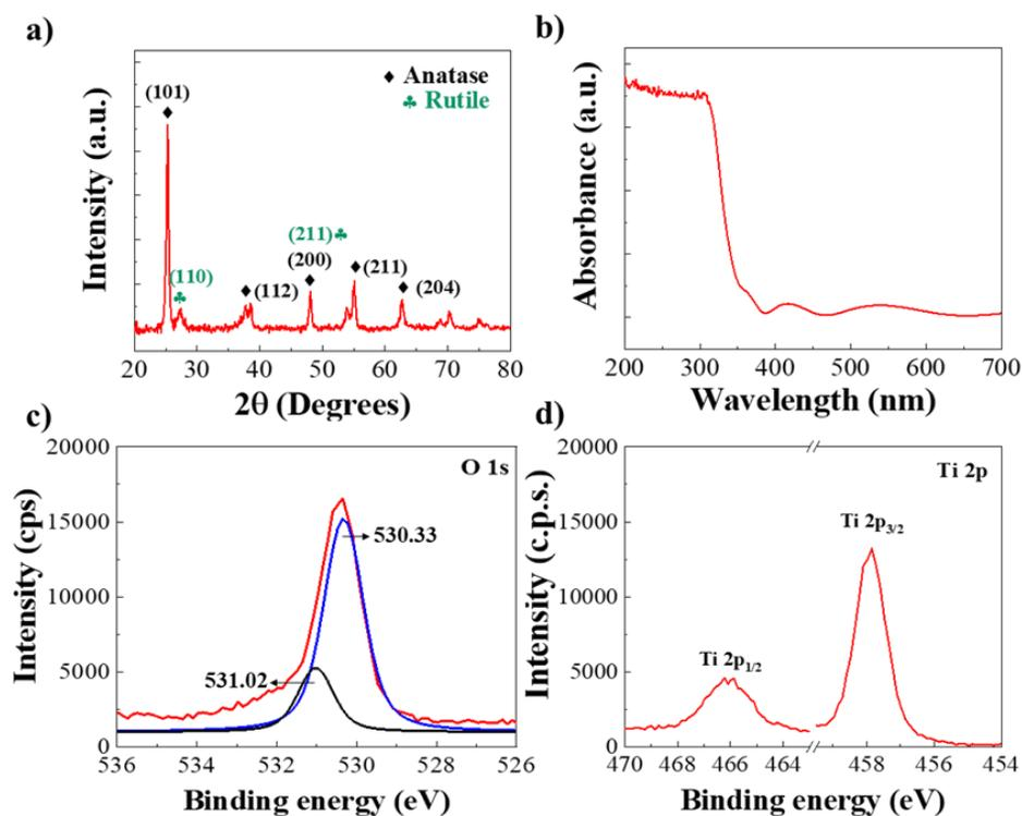
**Figure 7.** Characterization of a 270 nm sputter-deposited  $\text{TiO}_2$  film on a flat silicon substrate (samples A1-T2): (a) GI-XRD pattern, (b) UV-Vis absorption spectra (film deposited on quartz), XPS spectra, (c) O 1s, and (d) Ti  $2p_{1/2,3/2}$  regions.
