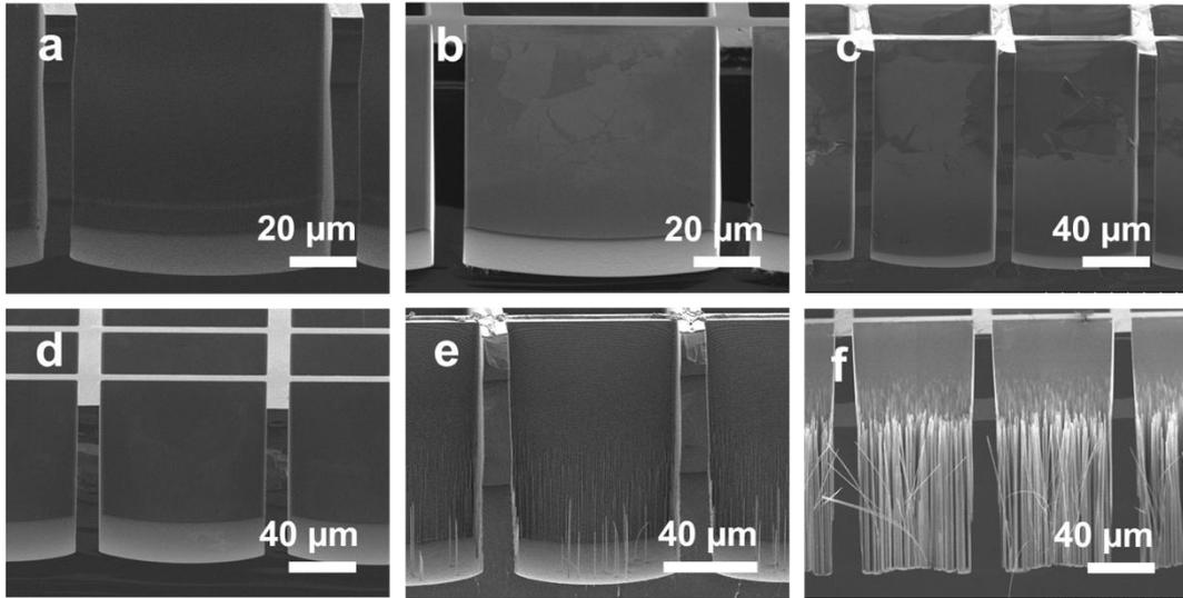
**Figure 5.** SEM cross-section images of silicon microstructures obtained by DRIE with  $SF_6:C_4F_8/O_2$  exposure time ratios of 1.67 (a), 1.10 (b), 0.85 (c), 0.75 (d), 0.57 (e) and 0.40 (f). The depths are 74  $\mu m$  (a), 75  $\mu m$  (b), 127  $\mu m$  (c), 75  $\mu m$  (d), 109  $\mu m$  (e) and 140  $\mu m$  (f).
