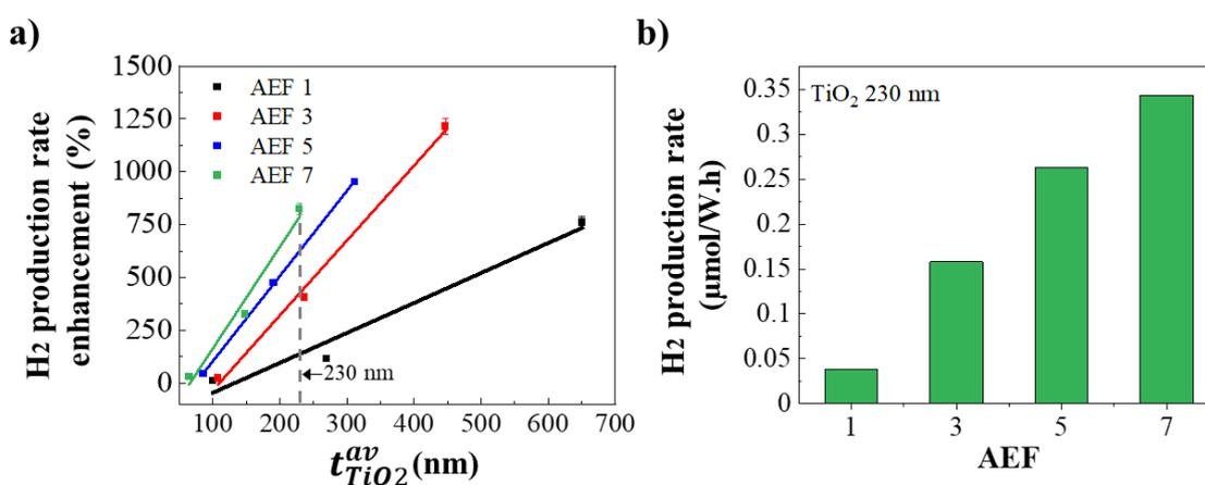
**Figure 9.** (a)  $\text{H}_2$  production rate enhancement as a function of the  $\text{TiO}_2$  average thickness ( $t_{\text{TiO}_2}^{\text{av}}$ ) for flat and 3D photocatalysts with AEFs of 3, 5 and 7. Values are compared to the  $\text{H}_2$  production rate of the reference sample A1-T2. Solid lines are obtained by linear regression.
