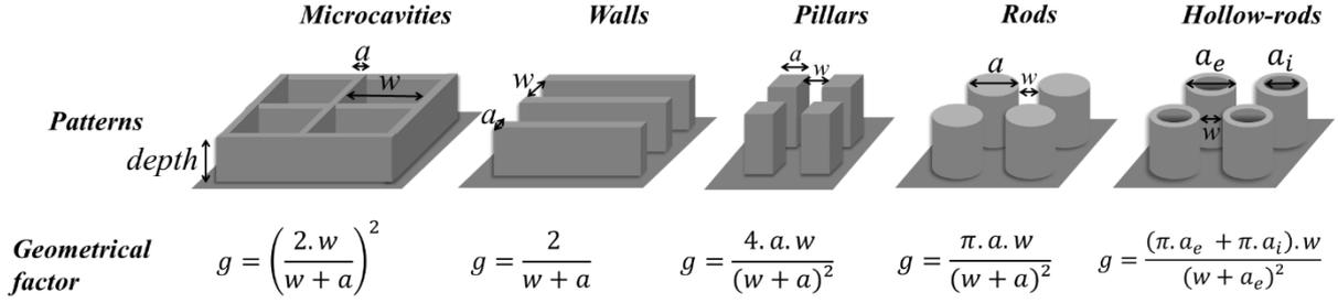
**Figure 3.** 3D view of the proposed patterns: microcavities, walls, square pillars, rods and hollow-rods, with their respective geometrical parameter  $g$  defined by the horizontal dimensions  $w$  and  $a$ .
