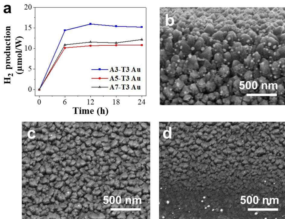
**Figure 10.** (a) Hydrogen evolution over 24 h for 3D photocatalyst composed TiO<sub>2</sub> and Au NPs featuring an AEF of 3,5 and AEF 7. SEM images of the top wall (b), wall at the half-height (c), and bottom wall (d) of the 3D photocatalyst TiO<sub>2</sub>/Au NPs labeled A3-T3.
