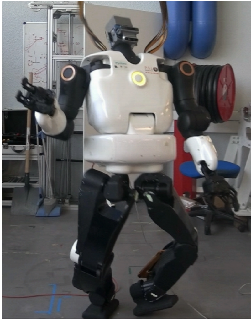
Figure 12. Failed experiment using torque control for a postural task.
