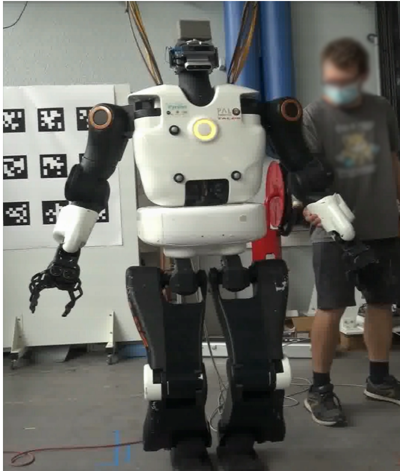
Figure 13. Successful experiment using torque control for a postural task.
