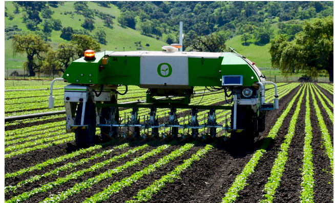
Figure 3: The Dino robot for vegetable weeding on large-scale vegetable farms. Source Naïo Technologies [10]
