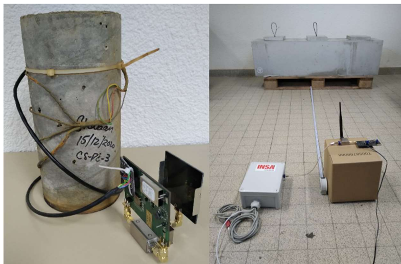
Figure 2. Photographs of: a sensing node with a resistivity sensor (left) and the experimental setup with sensing nodes embedded in a reinforced concrete beam (right).
