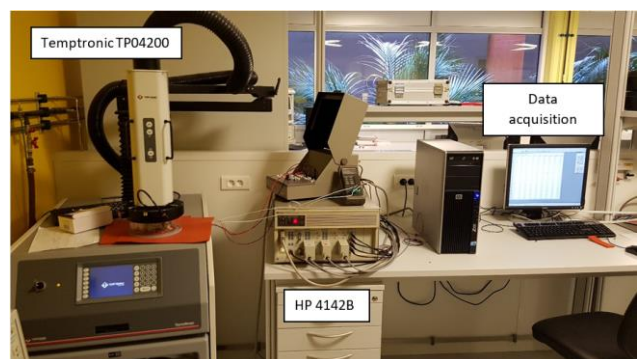
Fig. 3. Electrical test bench for power module characterization.
