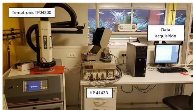
Fig. 3. Electrical test bench for power module characterization.
