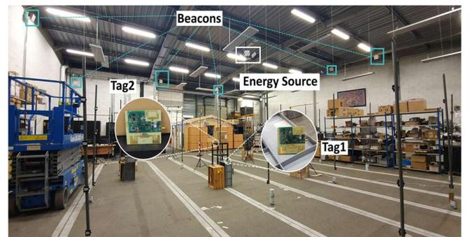
Fig. 7. Geolocation setup of the tags in the 300 m<sup>2</sup> test area. Thirteen beacons (only six are visible here) and two tags (placed at various position) have been used.
