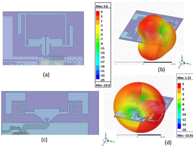
Fig. 3. Antenna design and simulation of the tag: (a) Proposed design of the UWB antenna; (b) 3D Radiation pattern of the UWB antenna at 4 GHz; (c) Proposed design of the UHF antenna; (d) 3D Radiation pattern of the UHF antenna at 868 MHz.
