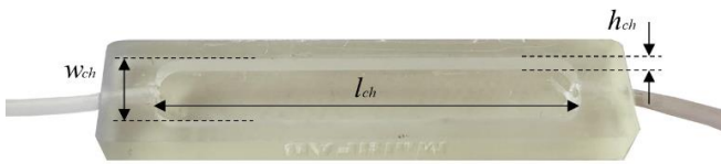
Fig. 4. Photograph of the designed fluidic channel including fluidic accessories. The dimensions of the fluidic channels are (in mm): l_{ch} = 35 , W_{ch} = 6 and h_{ch} = 2 .
