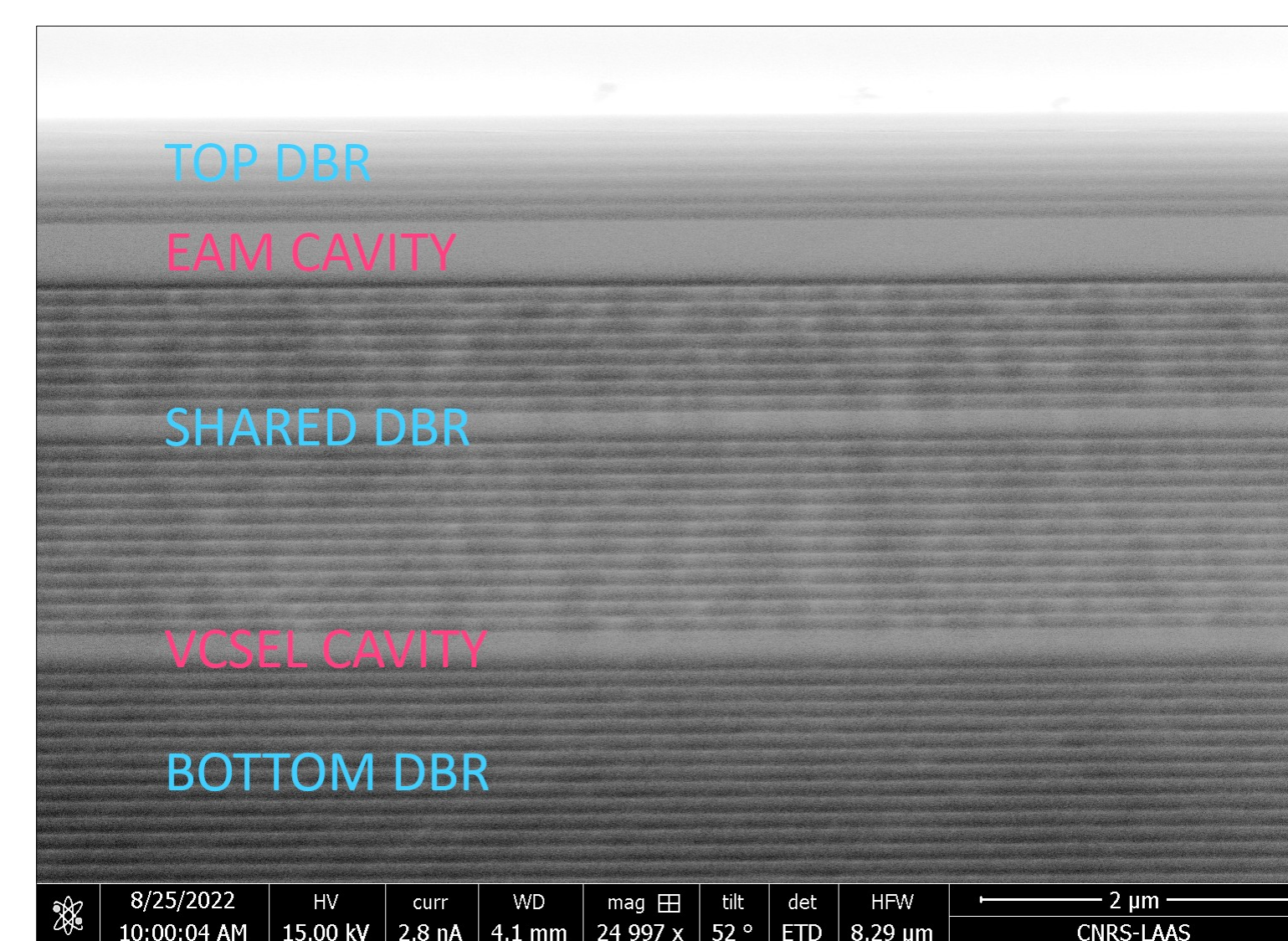
Scanning Electron Microscope cross-section view of the grown EAM-VCSEL structure
