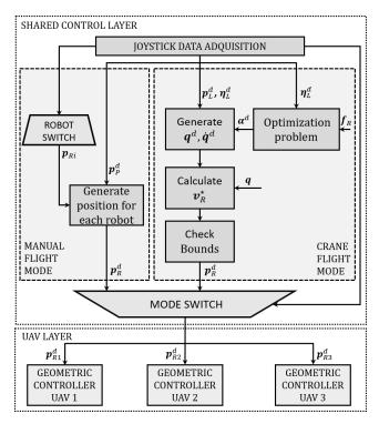
Fig. 5: Control strategy implemented for the G-Fly-Crane.
