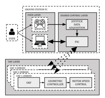
Fig. 4: Software Architecture.
