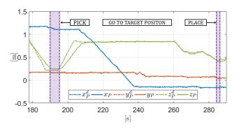
Fig. 7: Position Tracking for the operation of pick-and-place for the second brick.
