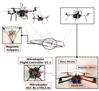
Fig. 3: G-Fly-Crane hardware scheme.
