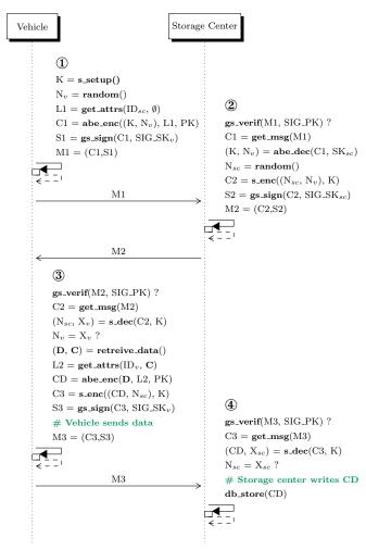
Fig. 2 Secure vehicle data send sequence diagram
