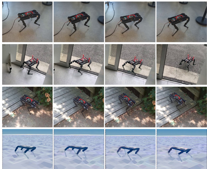
Fig. 1. Snapshots of the Solo12 quadruped in simulation and in real settings driven by a reactive controller learned through deep reinforcement learning. With learned controllers the robot can traverse various outdoor environments with slopes and rough ground. Full video: https://youtu.be/t-67qBxNyZI
