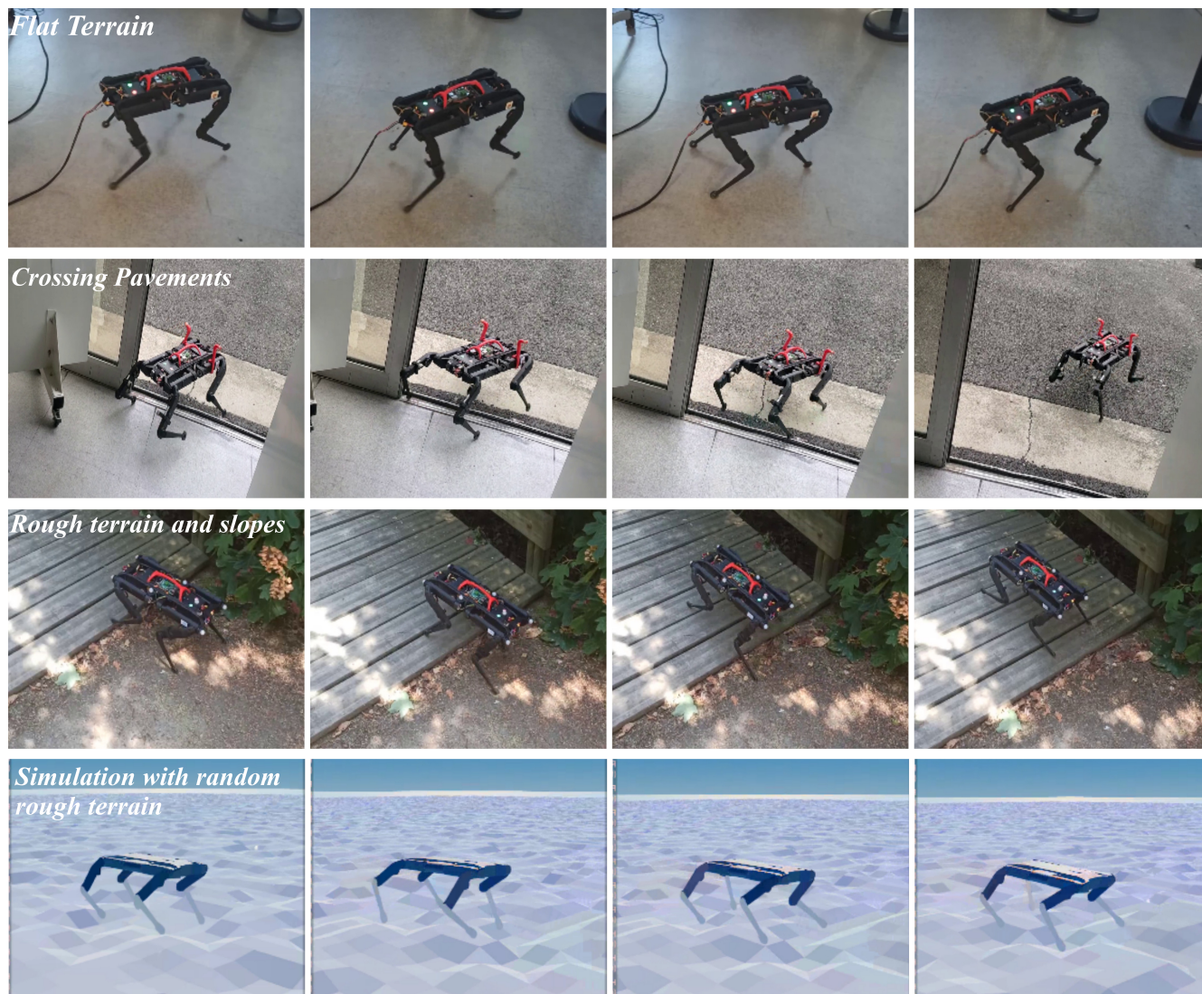
Figure 1. Snapshots of the Solo12 quadruped in real settings and in simulation driven by a reactive controller learned through deep reinforcement learning. With learned controllers, the robot can traverse various outdoor environments with slopes and rough ground, full video: https://youtu.be/t-67qBxNyZI
