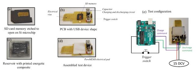
**Figure 6.** Photographs of (a) the SD card after being locally etched to reveal the silicon microchip that stores the sensible data, (b) the prepared SD card glued onto the demo PCB featuring a simple capacitive discharge circuit, (c) reservoir with printed energetic composite, (d) an assembled test device for demonstration tests, and (e) schematic of the demonstration test configuration.
