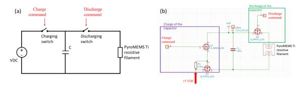
Figure 2. Design of the initiation unit: (a) schematic of the capacitive discharge circuit and (b) electronic circuitry with the discharge transistor (NMOSFET) shown in green and the charge transistors (NMOSFET + PMOSFET) shown in purple.
