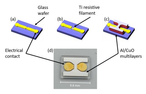
**Figure 3.** 3D schematic views of the main pyroMEMS fabrication steps: (a) Ti and Au deposition on a glass wafer, (b) etching of Au to define the electrical tracks and Ti resistance, (c) sputter-deposition of the Al/CuO multilayered reactive film, and (d) real view snapshot.
