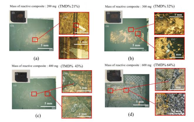
**Figure 8.** Photographs of SD cards after tests with energetic composite masses of (a) 200 mg or 90 mm<sup>3</sup>, (b) 300 mg or 130 mm<sup>3</sup> (c) 400 mg or 170 mm<sup>3</sup> (d) 600 mg or 268 mm<sup>3</sup> and with their insert (i) a global photograph of the SD card, (ii) microscope imaging with ×20 magnification and (iii/iv) microscope imaging with ×140 magnification.
