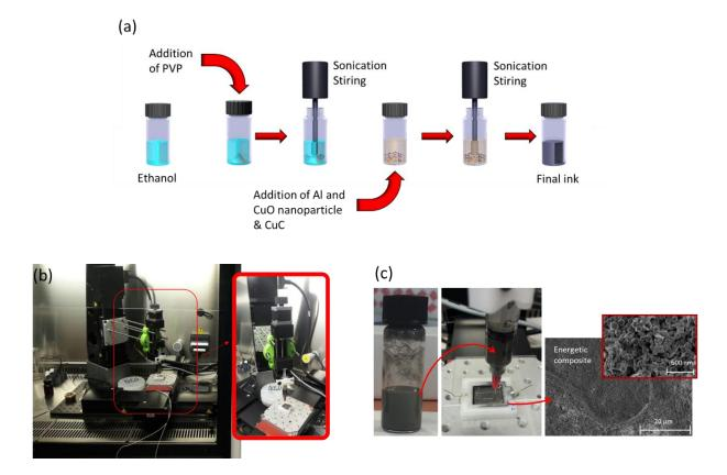
**Figure 4.** Energetic ink preparation and deposition: (a) schematic of the copper ammine complex and nanothermite ink preparation. (b) Photograph of the homemade 3D printer with the syringe driver pushing the syringe filled with energetic ink and the 3-axis controller.
