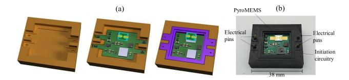
**Figure 5.** The USD packaging: (a) schematic of the 3 main parts of the USD with the external packaging in brown, the pyroMEMS in blue, the reservoir in which the energetic composite is printed in purple, and (b) a photo of the reservoir with the initiation circuit inside.
