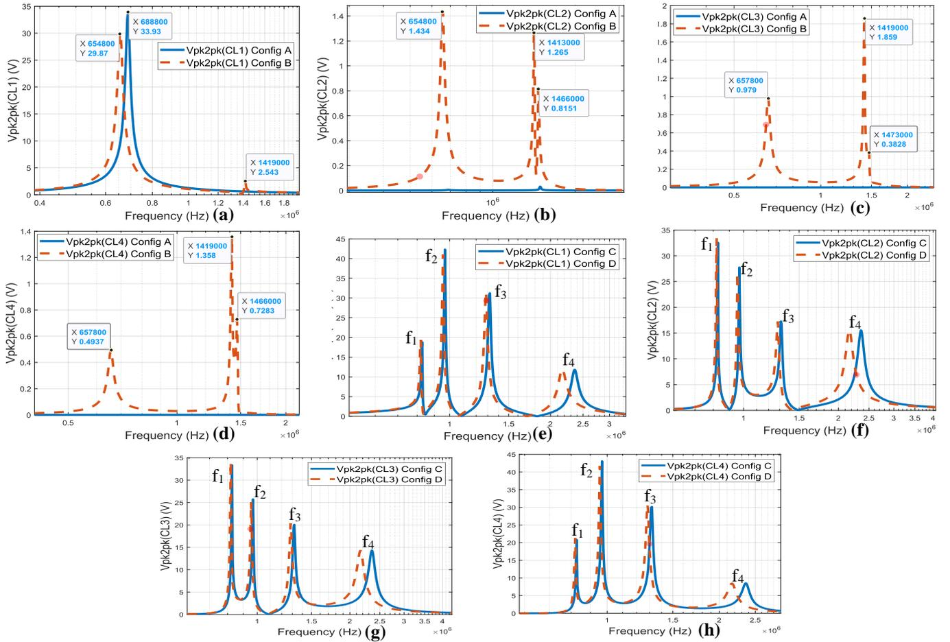
Fig. 5.  $V_{pk2pk}(C_{L_i})$  simulation results as a function of the injected frequency and comparing Config A with B and Config C with D. In the exception of the shown frequency range, the two curves of each graph fit together.
