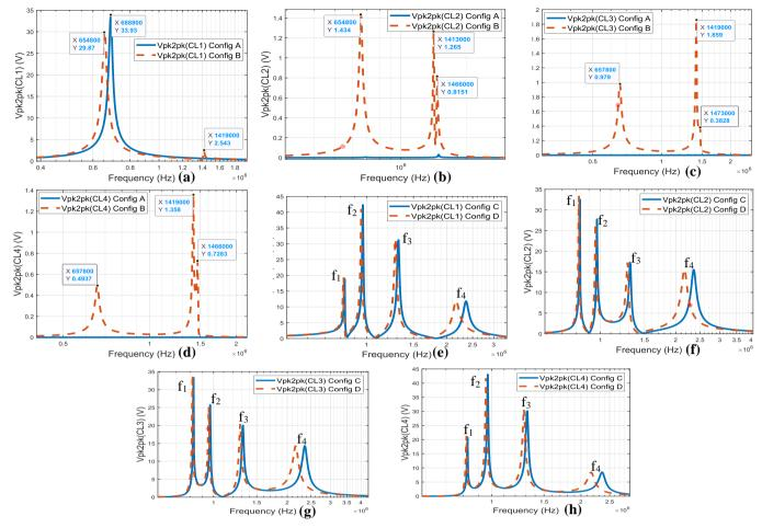
Fig. 5.  $V_{pk2pk}(C_{Li})$  simulation results as a function of the injected frequency and comparing Config A with B and Config C with D. In the exception of the shown frequency range, the two curves of each graph fit together.
