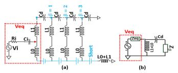
Fig. 6. Simplification of PCB model from Config C. (a) removal of  $C_L$  and  $R_b.$  (b) simplified model using  $Z_{\mbox{\scriptsize B}}$
