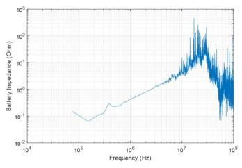
Fig. 3. Measured impedance profile of the battery from 150 KHz to 100 MHz.
