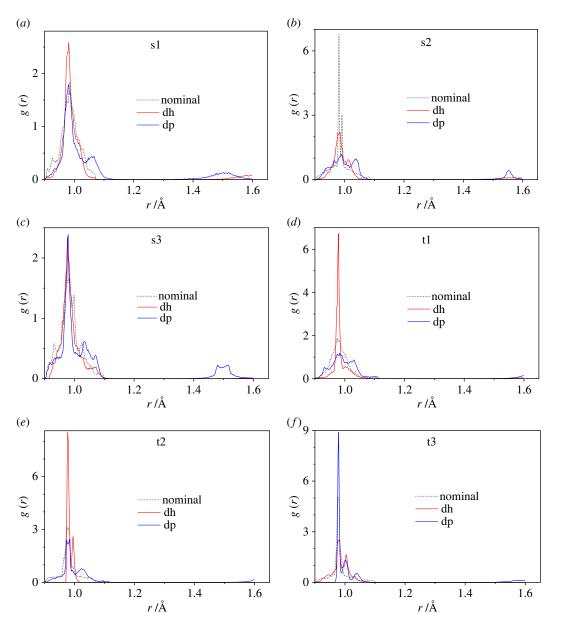
**Figure 15.** RDF g(r) of all hydrogen–oxygen atomic pairs for sucrose (*a*) s1, (*b*) s2 and (*c*) s3, and for trehalose (*d*) t1, (*e*) t2 and (*f*) t3, conformations for nominal (dotted black), dehydrogenated (red) and deprotonated (blue) modifications obtained using results of MD at the temperature of 40 K.
