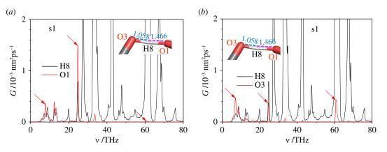
**Figure 18.** VDOS as function of frequency  $\nu$  of sucrose s1 (*a*) hydrogen atom H8 and oxygen atom 01, and (*b*) hydrogen atom H8 and oxygen atom 03 (only three atoms, H8, 01 and 03, were free to move during the MD).
