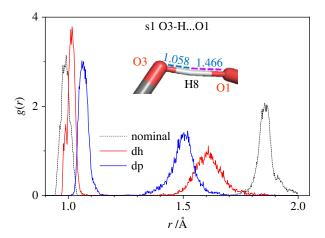
**Figure 16.** RDF g(r) of the atoms involved in the hydrogen bonding 03-H8...01 for nominal (dotted black), dehydrogenated (red) and deprotonated (blue) s1 sucrose modifications. Inset: fragment of deprotonated sucrose s1 atomic structure showing the hydrogen bonding 03-H8...01.
