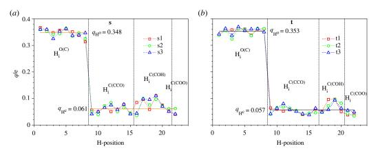
**Figure 4.** NAC (*q*) of hydrogen atoms for the nominal (*a*) sucrose and (*b*) trehalose molecules. The horizontal lines indicate the averaged NACs over three disaccharide conformations (s1, s2, s3; or t1, t2, t3) and hydrogen atom locations,  $H_i^{O(C)}$ ,  $H_i^{C(CO)}$ ,  $H_i^{C(COH)}$  and  $H_i^{C(COO)}$ .
