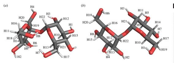
**Figure 1.** Nominal neutral (*a*) sucrose and (*b*) trehalose molecules. Hydrogen, carbon and oxygen atoms are represented by white, grey and red sticks, respectively.
