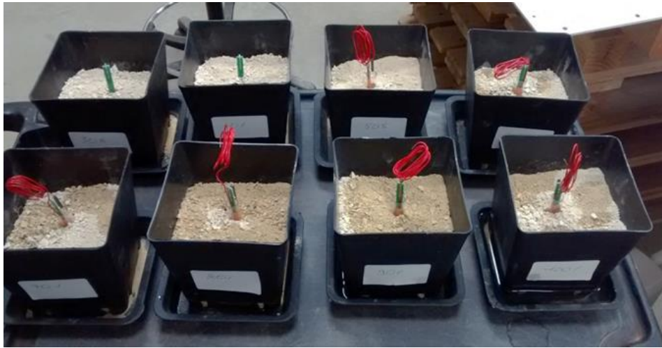
Figure 5: analysis of clay-silt soil matrices using ChemFET-based sensors
