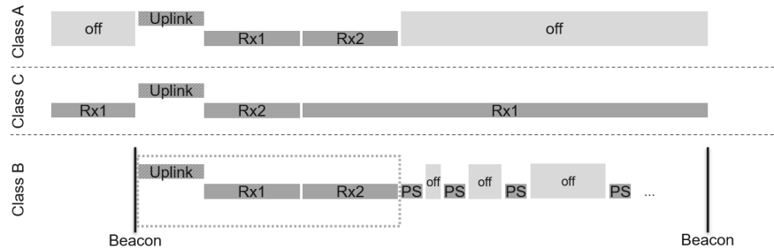
Fig. 1.7: The LoRaWAN communication mode: Classes A, B and C.
