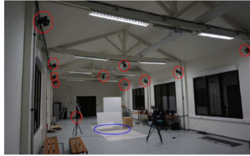
Fig. 2. CREPS laboratory. Cameras are indicated with the red circles and the three platforms with the blue circle
