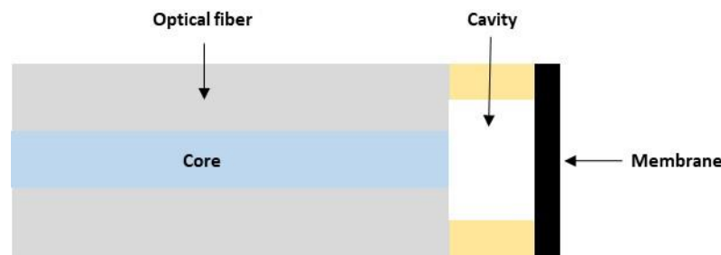
Figure 2. Topology of Fabry–Perot cavity sensor with a membrane as a mechanical transducer.
