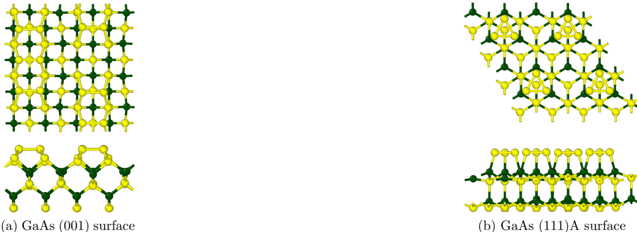
Figure 1: Top and side views of the supercells used for the modeling of (a) the GaAs (001) surface and (b) the GaAs (111)A surface. For clarity, only the topmost layers are represented. Yellow and green spheres represent As and Ga atoms, respectively.
