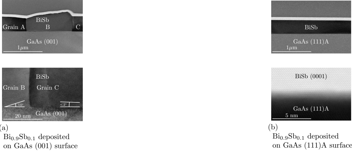
Figure 2: Transversal TEM images of the \text{Bi}_{0.9}\text{Sb}_{0.1} deposition on top of (a) the GaAs (001) surface and (b) GaAs (111)A surface.
