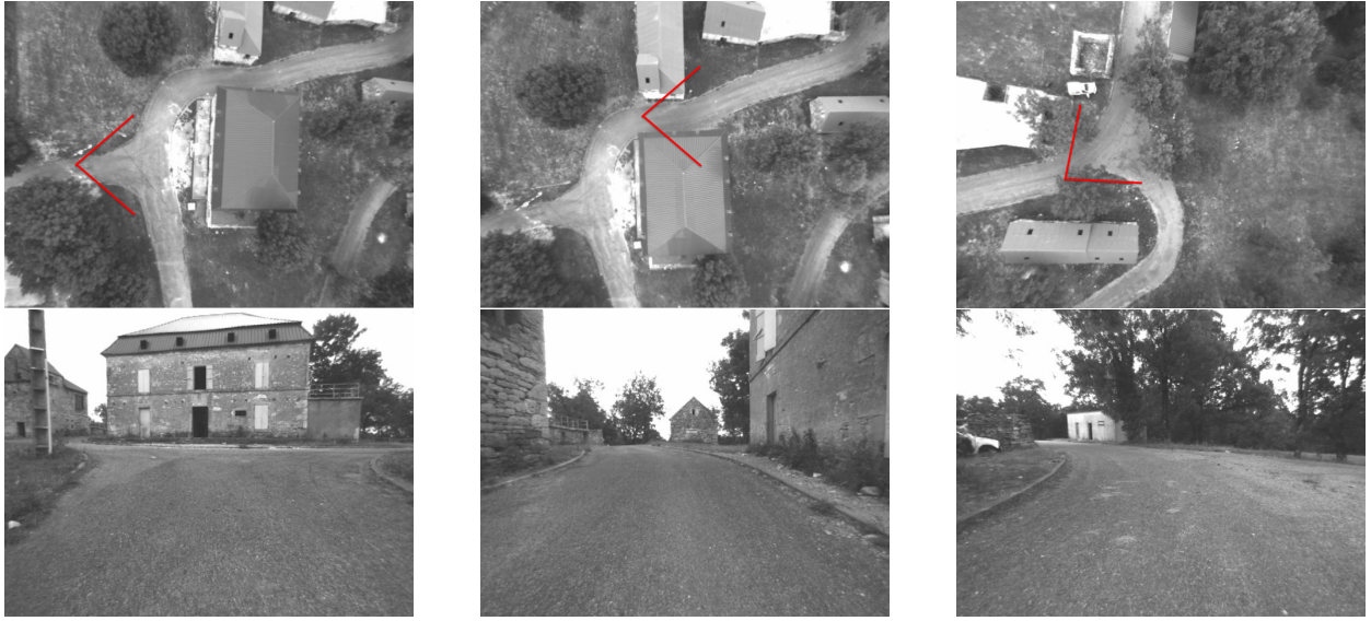
Figure 1: Three aerial images of a village acquired at about 40m altitude (top) and three images of the same area acquired by a ground rover. The red angular sector in the aerial images approximately represents the position and field of view of the ground rover camera. How could these data be registered and fused in a spatially consistent data structure?
