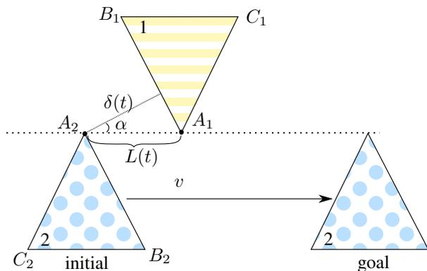
Fig. 5: Example of a single collision. Each body is a triangle  $A_iB_iC_i$ . Along the path, the triangle 1 (yellow stripes) is static. The triangle 2 (blue dots) moves from its initial position to its goal position with a constant velocity  $v$ . Along the path, the lines  $(B_1C_1)$ ,  $(B_2C_2)$  and  $(A_1A_2)$  are parallel. There is a single collision during the motion, which the algorithm generally fails to find.
