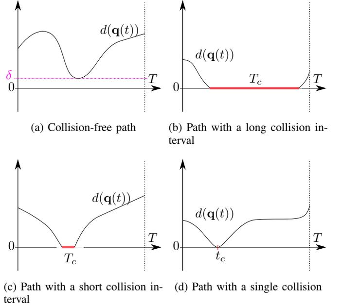
Fig. 3: Distance functions for four example paths
