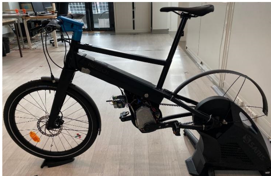
Figure 6. Experimental prototype e-bike mounted on the home trainer Saris.
