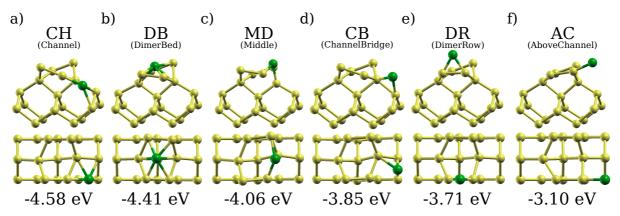
Appendix A. Stable adsorption sites of Ni on the Si (001) surface with their corresponding adsorption energies Eads. Yellow and green spheres represent Si and Ni atoms, respectively.
