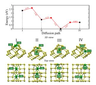
Figure 5: Most favorable insertion paths of two Ni atoms initially situated in DB configurations (from left to right) and insertion path of two Ni atoms initially situated in IDB + CH configuration (from right to left). Activation barriers (numerical values in red) are given in eV. An additional explored path is given in Appendix B.
