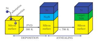
Figure 1: Schematic representation of the different stages needed to obtain NiSi silicide. The deposition of Ni atoms is first deposited with Physical Vapor Deposition (PVD) at ambient temperature forming an as-deposited interface of Ni3Si composition, which is then annealed at temperature below 700 K to form the targeted NiSi layer.
