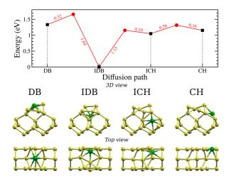
Figure 4: Insertion paths from DB (from left to right) and CH (from right to left) configurations into the topmost layers of the silicon substrate. The resulting configurations are labeled IDB (InsertedDimerBed) and ICH (InsertedChannel) 3D side and top views of each atomic configuration are provided. Activation barriers (numerical values in red) are given in eV.
