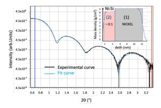
Figure 7: XRR profile of the as deposited sample. A schematic of the layered structure and obtained composition is provided in the inset: red area reveals a Ni:Si with a composition of 3:1. The blue curve represents the fit arising from the model which is in good agreement with the experimental data.
