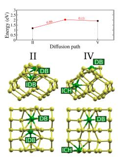
Appendix B. An additional explored path of the diffusion of two Ni atoms between an IDB+DB structure and an ICH+DB structure. This explored path indicates that it is not favorable for the Ni atom to diffuse far from the topmost layer at this level of coverage. Activation barriers (numerical values in red) are given in eV.
