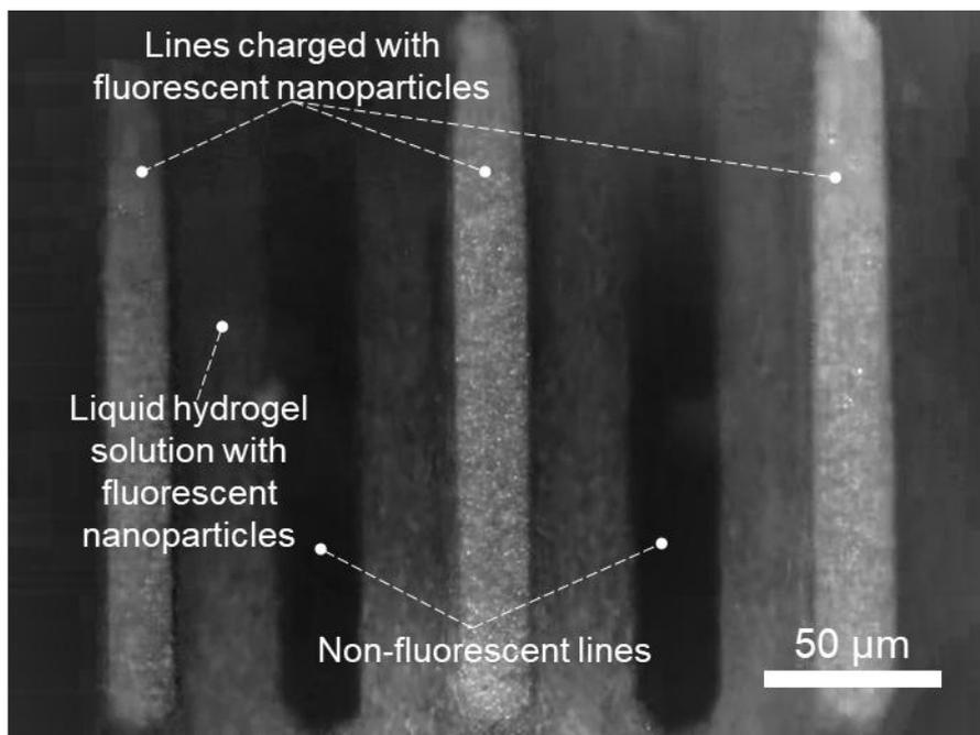
*Supplementary Figure 3. Optical image of 5 printed lines. The 1<sup>st</sup>, 3<sup>rd</sup>, and 5<sup>th</sup> contain nanoparticles visible under fluorescence, unlike lines 2 and 4. This picture was taken after printing but before rinsing, so we can see the nanoparticle-charged hydrogel material around the lines, which allows us to see the non-fluorescent lines by contrast. The printing video is available online.*
