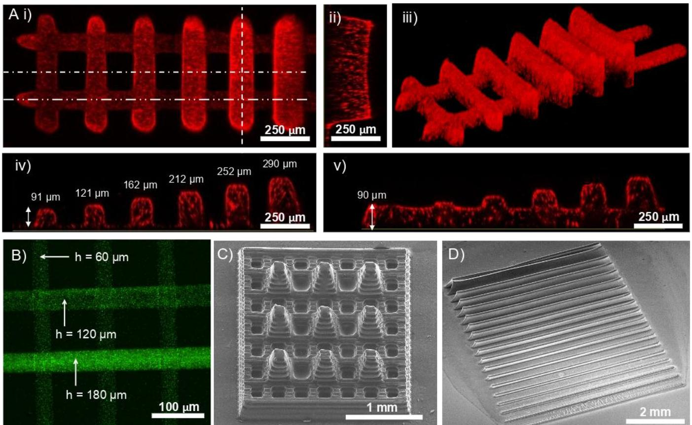
Figure 7. 2.5D and 3D PEGDA printed structures. (A) Confocal pictures of a ladder structure with segments printed at varying heights ( $h = 100$  or  $350 \mu\text{m}$ ). (B) Fluorescence image of crossing lines successively printed with three different printing heights. (C) SEM image of a millimetric 3D structure, including protruding and recessed pyramidal features. (D) SEM image of an array of lines with varying heights ( $h = 20\text{--}400 \mu\text{m}$ ).
