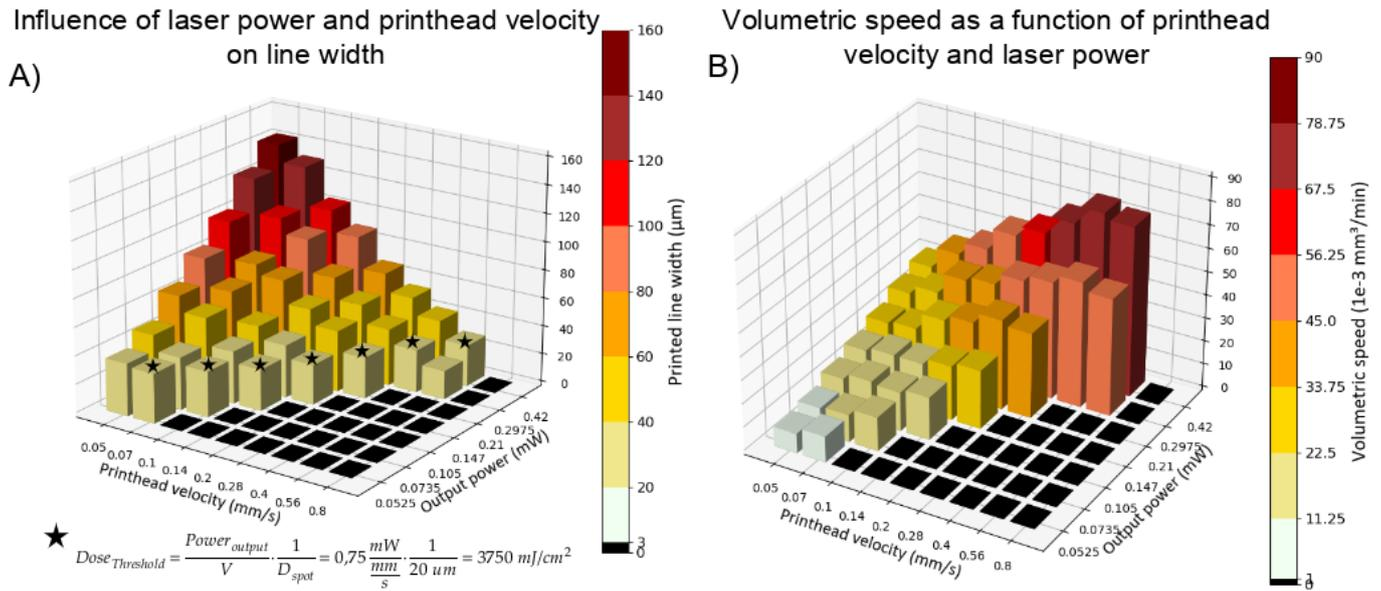
Figure 6. Study of the in-flow photopolymerization. (A) Influence of the optical output power and printing speed on line width. Experiment realized with  $h = 75$ ,  $\phi_{\text{in}} = 25 \mu\text{L}/\text{min}$ , and  $R\phi = 5$ . Dose threshold values correspond to the minimum dose giving rise to stable structures (marked with a  $\star$ ). (B) Volumetric printing speeds based on the data in Fig 6.A data and eq. 4.
