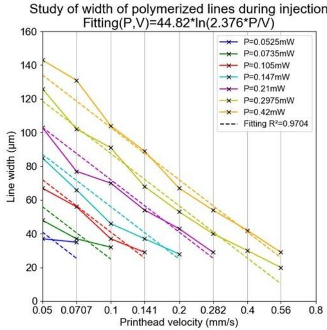
Supplementary Figure 6. Experimental results for the influence of the input power and printhead velocity on the printing line width.  $h = 75 \mu\text{m}$ ,  $\varphi_{in} = 25 \mu\text{L}/\text{min}$  and  $R\varphi = 5$ . Fitting realized with eq. 3:  $Width(P_{out}, V) = k_1 \cdot \ln(k_2 \cdot P_{out}/V)$ , with  $k_1 = 44.82$ ,  $k_2 = 2.376$ .
