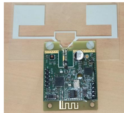
Fig. 4. Electrical schema of the BFSN and a photo of the manufactured of battery-free SN prototype including a flexible antenna manufactured on PET substrate operating in ISM 868 MHz frequency band.
