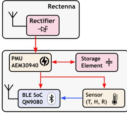
Fig. 2. Bloc diagram of the battery-free SN
