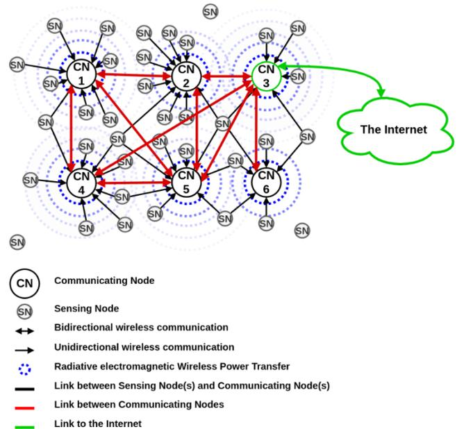
Fig. 1. Topology of the mesh network including battery-free SN.
