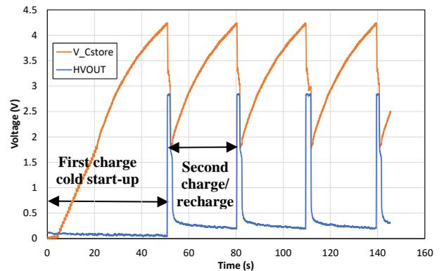
Fig. 7. Measured voltage at the input port of the storage capacitor ( $V_{Cstore}$ ) and at the output of the power management unit ( $HVOUT$ ) as function of time. Experimental results obtained by using the setup represented in Fig 6 b) for a RF power at +6 dBm delivered by the RF generator and injected to the rectifier input of the BFSN.
