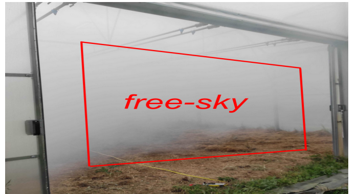
(b) Example of smoke dissipation performed by opening the rear-doors. Note that the smoke is not uniformly distributed in the chamber during dissipation and evacuates mainly by the top of the chamber.
