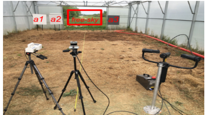
(a) Sensors and targets layout in the artificial fog experimental setup. At the rear-side of the chamber are disposed the a1 , a2 and a3 targets in this order (decreasing reflectivity order). At the entrance, from left to right : the PSD sensor, the OS1-128 LiDAR, a Biral VPF700 scatterometer and the smoke machine.
