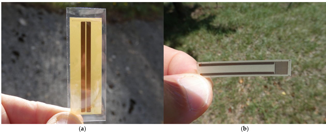
Figure 3. Examples of (a) 25 Ω Vishay T gauge and (b) 48 Ω Vishay longitudinal gauge.
