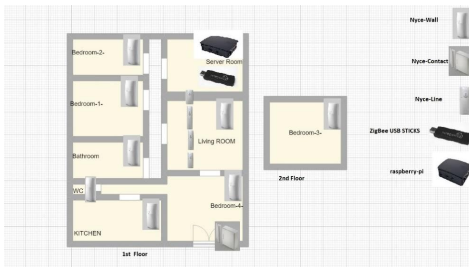
Figure 3. Architecture for the house
