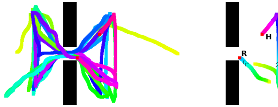
Fig. 7. Execution of the long run scenario using the TDP robot planner and InHuS. We see the complete set of time-colored paths on the left. On the right, the same path is cut, around the moment when the robot got stuck in the wall.
