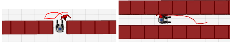
Fig. 4. In the doorway scenario (left), the reactive-only (Pedsim) agent never stops moving while trying to go through the robot even though its path is blocked. In the narrow corridor scenario (right), the agent squeezes itself between the wall and the robot colliding with both.
