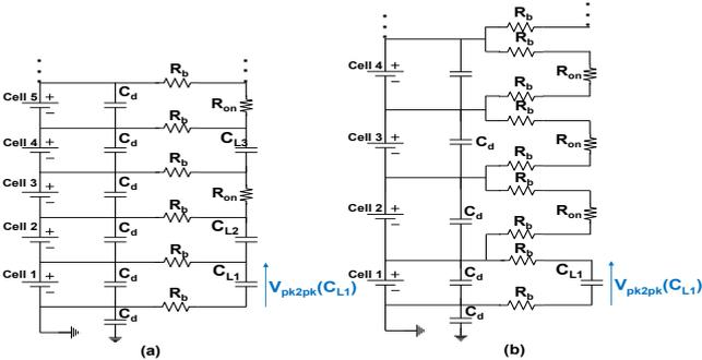
Fig. 4. First balancing approach on architecture 1 and architecture 2.
