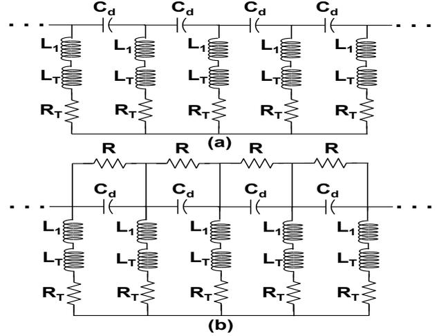
Fig. 7. Considered scenarios to analyze the impact of cell balancing on injection levels. (a) without balancing. (b) with balancing.
