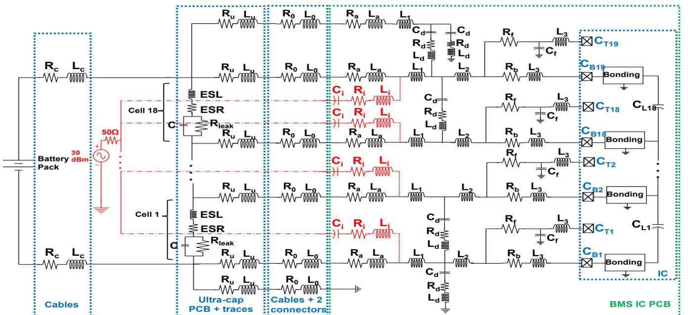
Fig. 2. Modeling of Architecture 1 of the BMS IC and its environment during DPI tests.
