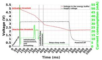
**Fig. 4.** Example of the power consumption of the sensing nodes according to the phase of operation.
