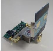
**Fig. 11.** Photographs of prototypes of the sensing nodes, using or not the Printed Circuit Board as a 6 cm x 8 cm metallic reflector plane located at 5 cm below the unique antenna.
