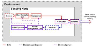
Fig. 2. Bloc diagram of the proposed generic architecture of the Sensing Node.
