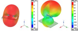
**Fig. 7.** Simulated (HFSS) radiation patterns of the printed folded quart-wavelength dipole antenna with capacitive arms at 868 MHz, with and without the use of a 6 cm x 8 cm metallic reflector plane located at 5 cm below the antenna/rectenna.
