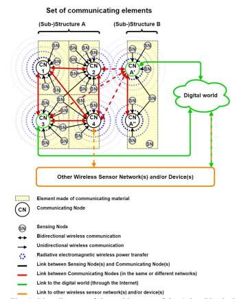
**Fig. 1.** Bloc diagram of the architecture of the Cyber-Physical System dedicated to the implementation of communicating materials.
