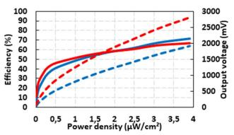
Fig. 9. Computed efficiency (full lines) and measured output DC voltage (dashed lines) against power densities for the printed folded quart-wavelength dipole rectenna with capacitive arms without (blue) and with (red) the use of a 6 cm x 8 cm reflector plane located at 5 cm below the antenna/rectenna, at 868 MHz and for a 10 k $\Omega$  resistive load.
