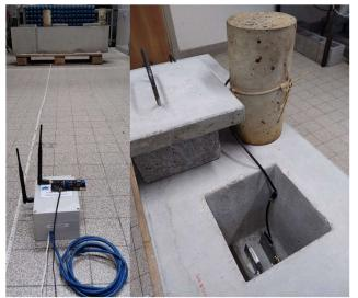
**Fig. 20.** Photographs of a complete Cyber-Physical System composed of 3 Sensing Nodes embedded in a reinforced concrete beam, and of 1 Communicating Node.
