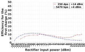
**Fig. 18.** Energy efficiency of the Sensing Nodes during the first charge against the conducted electromagnetic input power applied at the input of the rectifier, for a frequency of 868 MHz, and for two configurations of the wireless communication: transmission power of +4 dBm and data-rate of 5470 bps (blue), and transmission power of +14 dBm and data-rate of 250 bps (red).
