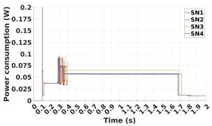
**Fig. 16.** Power consumption of the Sensing Nodes for a transmission power of +14 dBm and the slowest data-rate (DR0).
