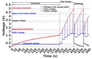
**Fig. 10.** Voltages, during a cold-start, a complete first charge and then a recharge, at the input of the Texas Instruments BQ25504 Power Management Unit (blue), in the energy buffer (red), and at the output of the Texas Instruments TPS63031 DC-to-DC buck-boost converter (black), for an input power of +0 dBm at 868 MHz.
