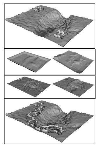
Figure 8: a/ the terrain model and the initial/final configurations. b/ the associated cost and potential functions. c/ the  $S_{\varphi}$  surfaces for  $\theta = 0$  and 90deg.. d/ the trajectory found by the planner
