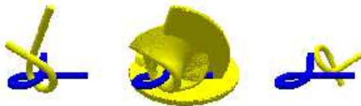
Figure 1. How to disassemble yellow and blue parts? This is a path planning problem.
