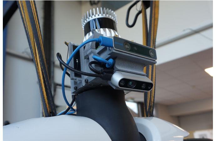
Fig. 1: New experimental head of the TALOS robot, with the D435i on the bottom, the T265i in the middle and the OS1-64 LiDAR on the top.
