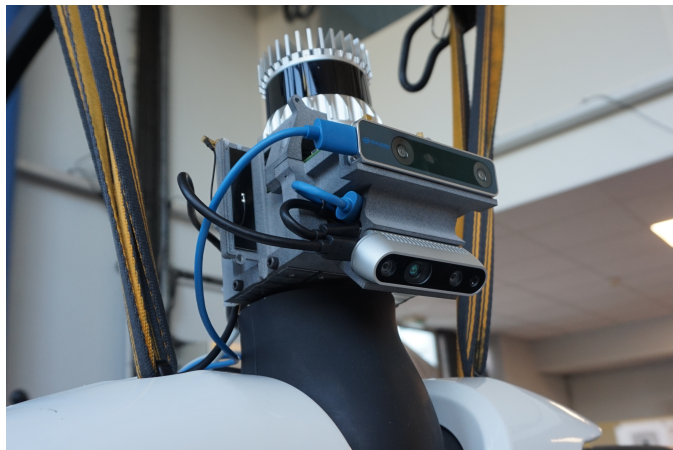
Fig. 1: New experimental head of the TALOS robot, with the D435i on the bottom, the T265i in the middle and the OS1-64 LiDAR on the top.
