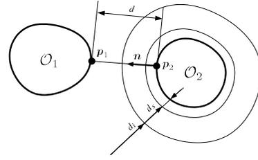
Fig. 2. Collision avoidance: Faverjon and Tournassoud's method
