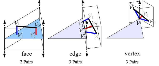
Fig. 3. Constraints generated between an edge and a triangle
