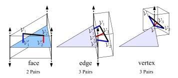
Fig. 3. Constraints generated between an edge and a triangle
