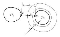
Fig. 2. Collision avoidance: Faverjon and Tournassoud's method
