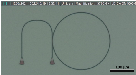
Fig. 3: Microscope image of the fabricated \text{Si}_3\text{N}_4 MRR.
