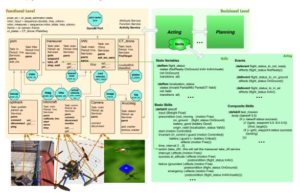
Figure 7: Architecture of the drone experiment.
