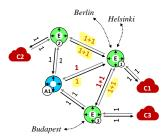
Figure 4: Aggregated topology with non-border node.
