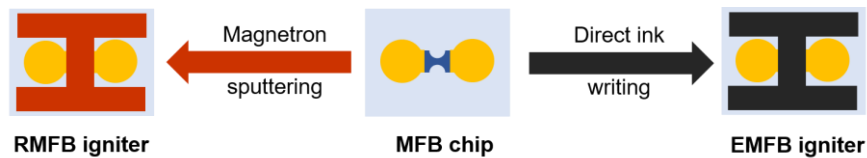
Figure 3. Schematics of the energetic layer deposition, by magnetron sputtering and direct ink writing, to achieve a high-energy and low-power MFB igniter.
