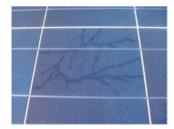
Fig. 1. Example of snail trail fault. Note the visual similarity with the trail of a snail.
