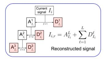
Fig. 5. Decomposition into 3 levels applied on the current signal  $I_i$  of each faulty or healthy panel.
