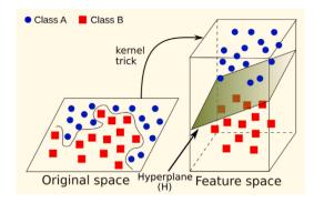
Fig. 8. Example of classification hyperplane representation of SVM.  ${\cal H}$  corresponds to the optimal hyperplane.
